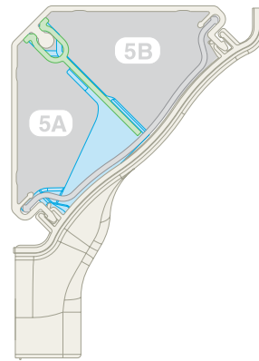
Cable fill #5: Divided channel (power and data) with low profile transition insert.
